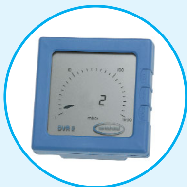
Vacuum gauge DVR 2 for the measuring range 1080 - 1 mbar with integrated capacitance pressure transducer
